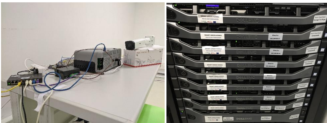
FIGURE 32: EFACEC_E-UC1 – SECONDARY SUBSTATION AUTOMATION IN IT LAB AND CONTROL CENTER SOFTWARE IN DATACENTER
