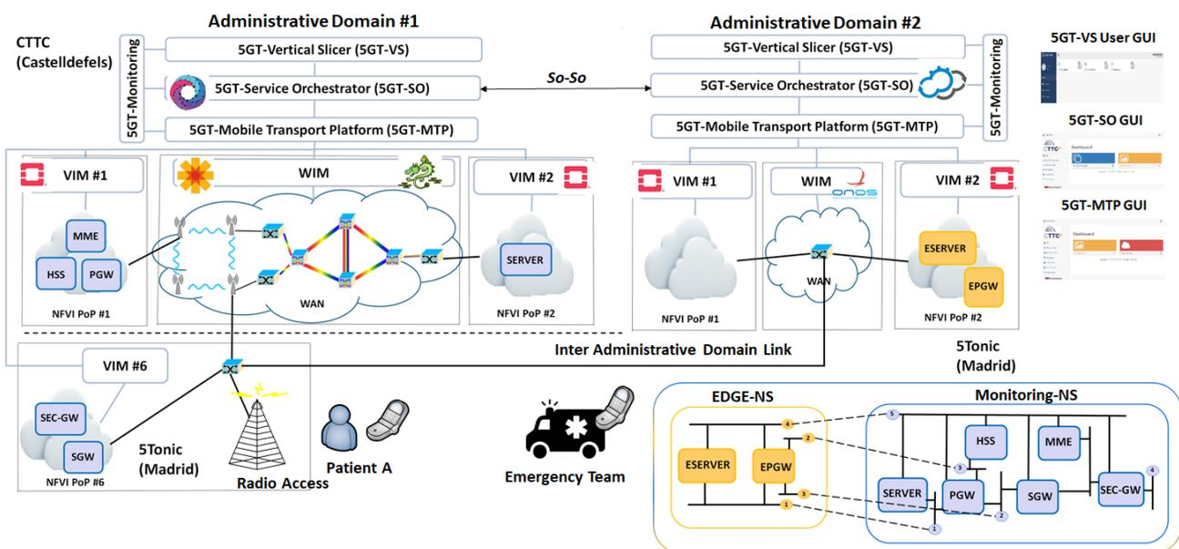
FIGURE 4: SETUP UNDER DEMONSTRATION FOR THE NFV SERVICE FEDERATION DEMO
