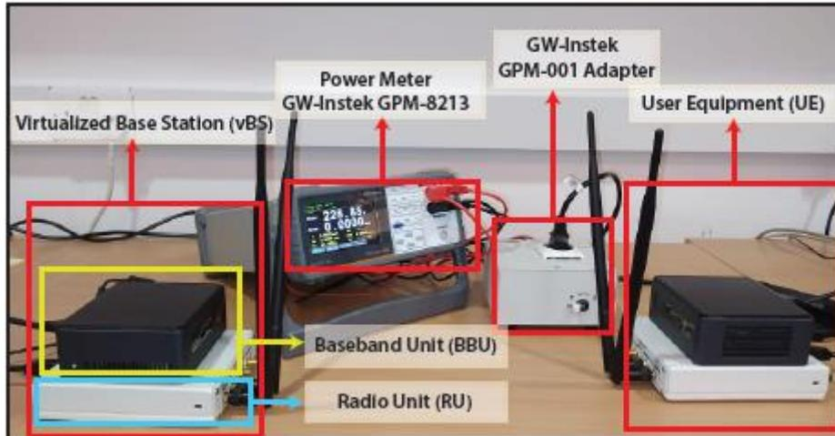
FIGURE 25: EXPERIMENTAL VBS AND UE TESTBED.
