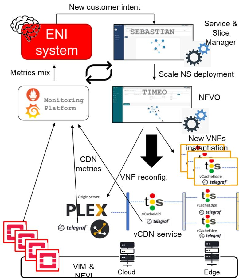
FIGURE 15: SYSTEM ARCHITECTURE OF ENI POC #9
